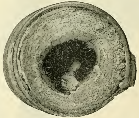
End view of hose made by competing company, wire-wrapped, showing inside diameter decreased to one-half its normal size. Cause—cheap material, and wire wrapping contracting it and not allowing it to expand.
